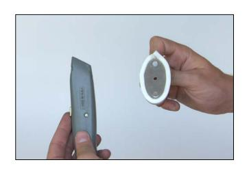
6) Once the adhesive strip is secure to the outside edge, use a utility knife to trim away two slots in the adhesive strips. This will allow for the glue to travel underneath the entire mount.
