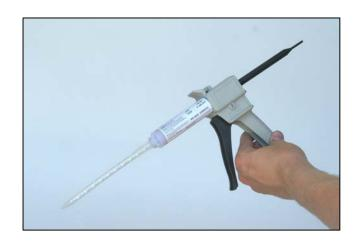
10) This is how the adhesive gun should look when assembled. Once it is assembled, cut the first notch off of the mixing nozzle using a utility knife.
