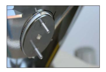
14) The mount must be undisturbed for 24 hours to allow for curing. Once the adhesive has cured, use a utility knife to trim off the excess adhesive. This is how the Stick & Shake mount™ should look once completed.
