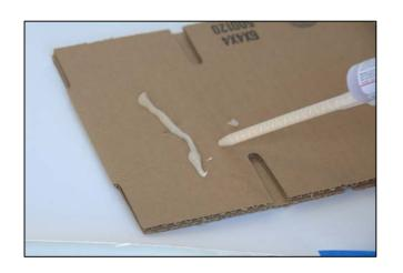
11) Squeeze the trigger until adhesive comes out of the mixing nozzle, and then squeeze out an additional 3" line to ensure a proper mixture is acquired.
