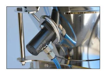
15) The vibrator can now be fastened onto the mount and used. This is how the Stick & Shake™ mounting system looks with the NTP 18 attached to it.
