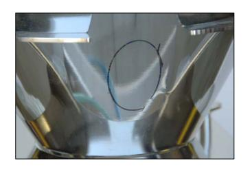
4) Remove the mount from the hopper/bin to ensure that a visible outline has been created.
