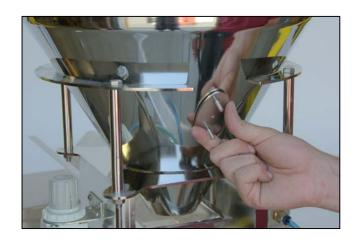
2) Position the mounting plate 1/3 up the sloped section of the hopper/bin. Note: Flat surfaces or curved surfaces with a minimum diameter of 8 inches.
