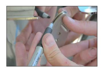
3) Using a marker, trace around the outside edge of the mount.
