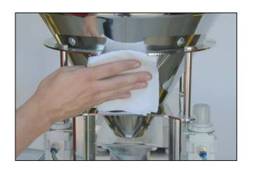
1) Clean the hopper/bin using a towel with wax and grease remover to allow for a clean working area.
