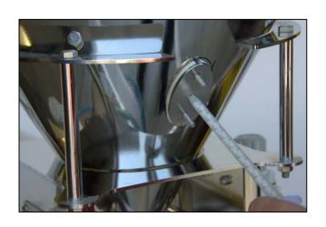
12) Insert the tip of the mixing nozzle into one of the open holes on the mount bracket as shown on the left.
