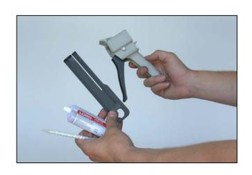
9) Acquire all of the components in the picture to the left to assemble the adhesive gun.
