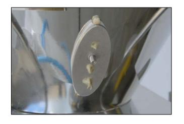
13) Squeeze the trigger on the adhesive gun until adhesive comes out of all the open holes and ends of the mount to ensure the proper amount of adhesive.
